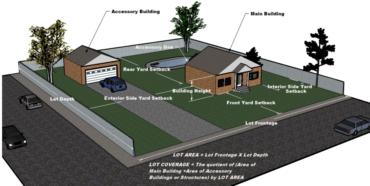
Figure 3.1: Main Building and Accessory Building
