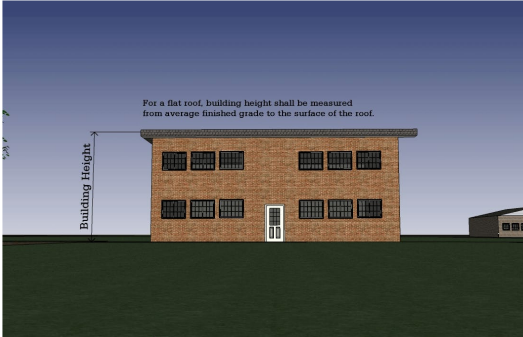
Figure 3.11: Building Height with Flat Roof
